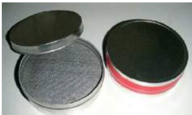
Fig. 3 - Canestro al carbone attivo (da www.researchgate.net/publication/239815223_Radon_adsorbed_in_activatd_charcoala_simple_and_safe_radiation_source_for_teaching_practical_radioactivity_in_schools_and_colleges/figures?lo=1 ).
